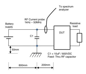
Test set-up conducted emission, power lead
