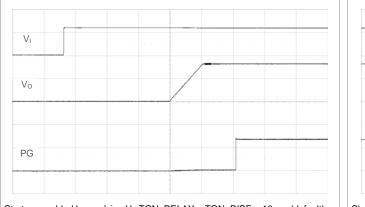
Start-up enabled by applying V<sub>I</sub>. TON\_DELAY = TON\_RISE = 10 ms (default). V<sub>I</sub> = 12 V, I<sub>o</sub> = max I<sub>o</sub> PG pulled up to V<sub>o</sub>. Scale: 10 or 2 V/div, 10 ms/div.
