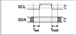
Setup and hold times timing diagram
