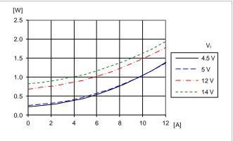
Dissipated power vs. load current and input voltage.
