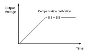
By the PMBus command ADAPTIVE\_MODE the user may select between several different modes of compensation calibration:
