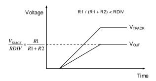
Ratiometric Voltage Tracking
