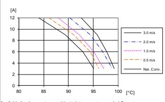
Available load current vs. ambient air temperature and airflow at  $V_1 = 12$  V. See section Thermal Consideration.
