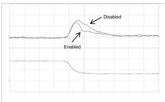
V<sub>I</sub>=12 V, V<sub>O</sub>=0.6 V, C<sub>O</sub> = 3x100 μF + 270μF/10mΩ, load step 3-9-3 A,1 A/us. FEEDBACK\_EFFORT = 0.8, ZETAP = 1.5. Scale: 20 mV/div, 5 A/div, 10 µs/div.
