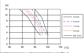
Available load current vs. ambient air temperature and airflow at V<sub>I</sub> = 12 V. See section Thermal Consideration.
