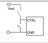
The product is equipped with a remote control function, i.e., the CTRL pin. The remote control can be connected to either the primary negative input connection (GND) or an external voltage (Vext). See Absolute Maximum Rating for maximum voltage level allowed at the CTRL pin.
