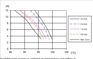
Available load current vs. ambient air temperature and airflow at  $V_1 = 12$  V. See section Thermal Consideration.
