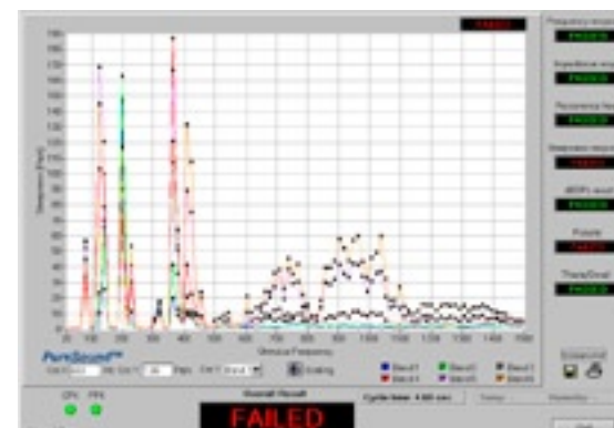
Rub&Buzz Test Result, Loose Particle in Driver
