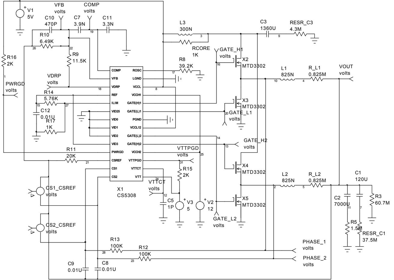
**Figure 5.4.1: 5V to 1.7V/ 28A at 335kHz with 12V Bias
