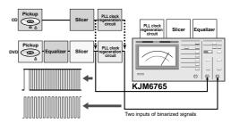
Note: To measure a binarized signal, the SYMMETRY mode of the KJM6765 must be set to MANUAL.
