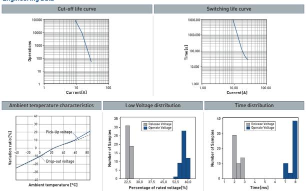
**Note** : I-T curve at ambient temperature of 23  $^{\circ}$ C
